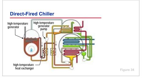
The **high-temperature generator pump** draws a portion of the intermediate solution from the low-temperature generator and delivers it to the high-temperature generator to be reconcentrated.
